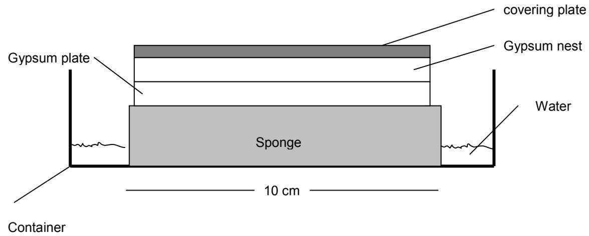
Figure 4. Experimental Set up Gypsum nest, side view (Umweltbundesamt 2001)
