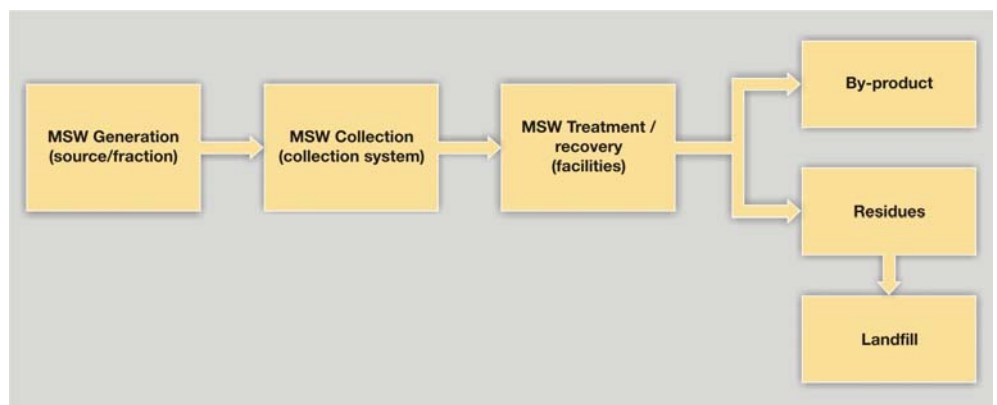
Figure 1 Generalised waste flow
