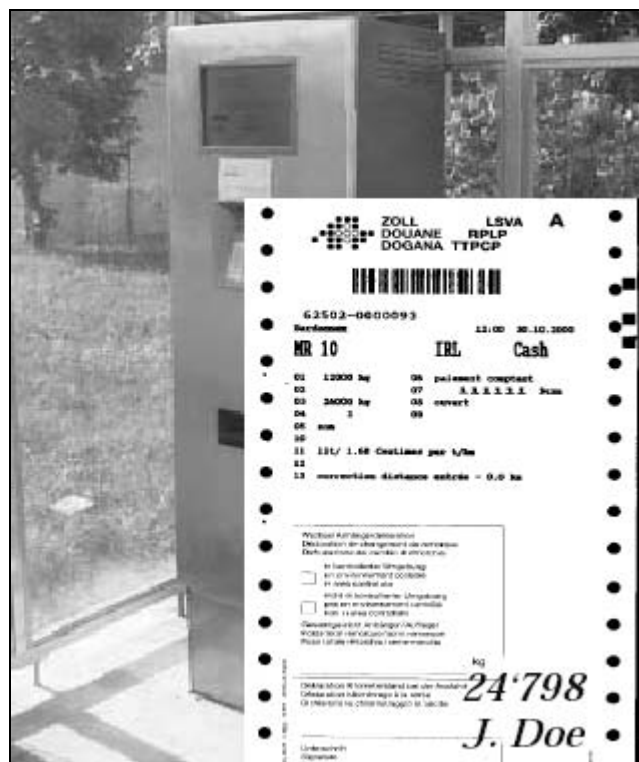
Figure 3. Clearance terminal for users without OBU
