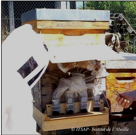
Capture at the hive entrance Hive is equipped with a RFID system (Microsensys, GmbH, Erfurt, Germany)
