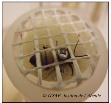
RFID tag glued on the bee thorax with glue (dental cement, Temposil®)
