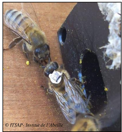
Tagged bee on the flight board RFID reader with tunnel to scan labelled bees going in and out the hive
