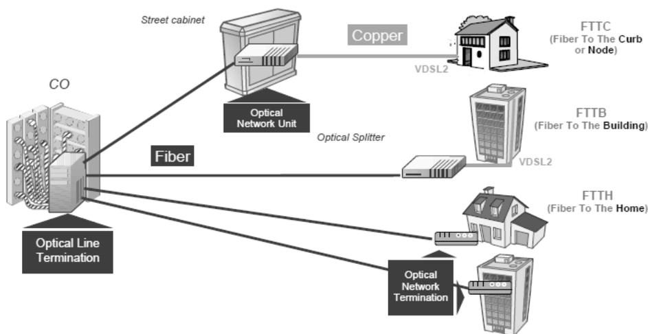
**Figure 8: A Point-to-Multipoint fibre deployment**
