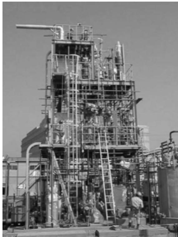
**Figure 2 Pilot plant of decomposition of dioxin by SCWO**
