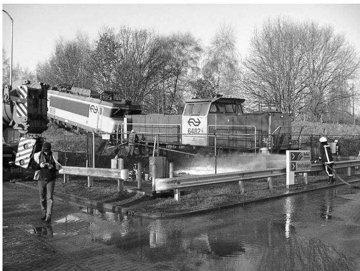
Image: In Arnhem, Netherlands, a LPG tankstation was located next to an up-level marshalling yard / freight station in a densely populated area. In the shunting process some wagons were incidentally pushed off the marshalling yard and nearly hit the LPG stationary below the shunting yard.
