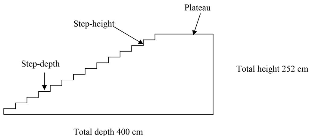
The diagram below illustrates a staircase with 14 steps and a total height of 252 cm:
