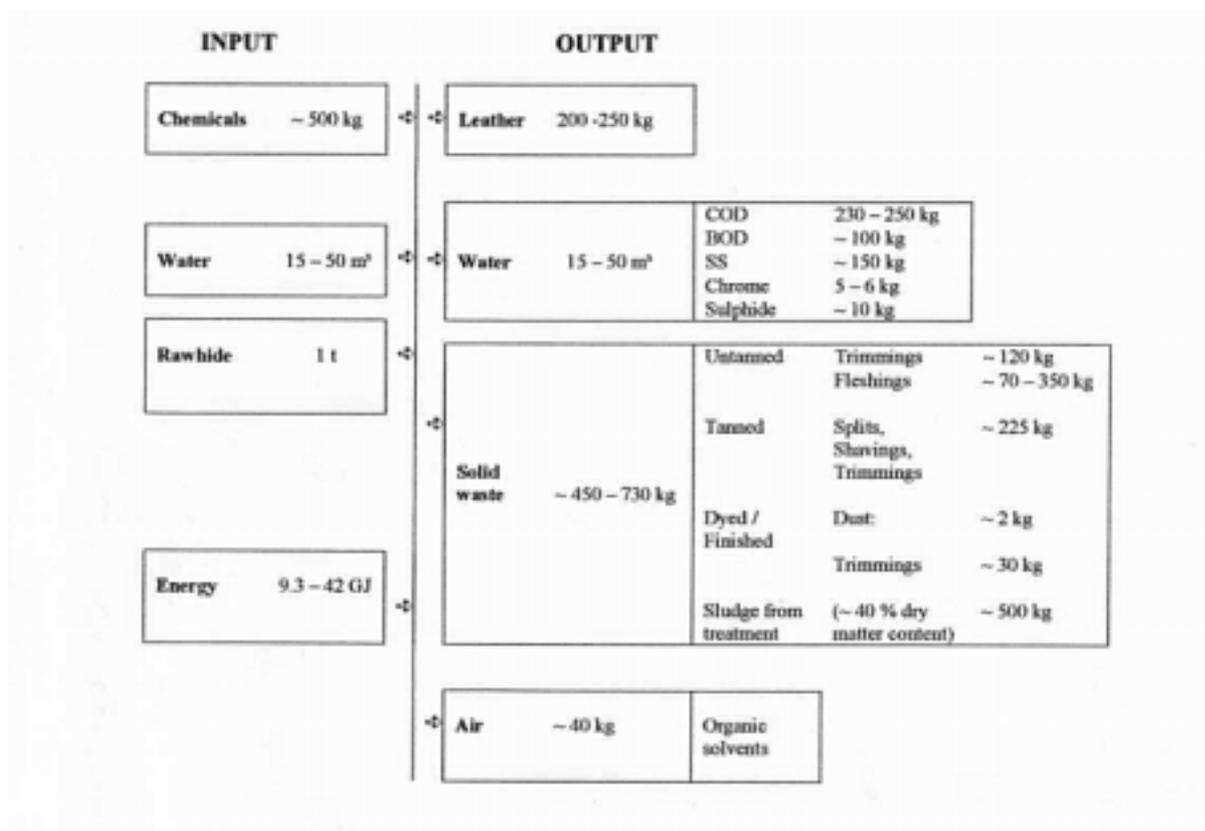
Figure 1 Input\* and output overview for chrome-tanning of 1 tonne salted bovine hides (BREF 2003, p. 5); \* = 500 kg chemicals input include approx. 200 kg curing salt
