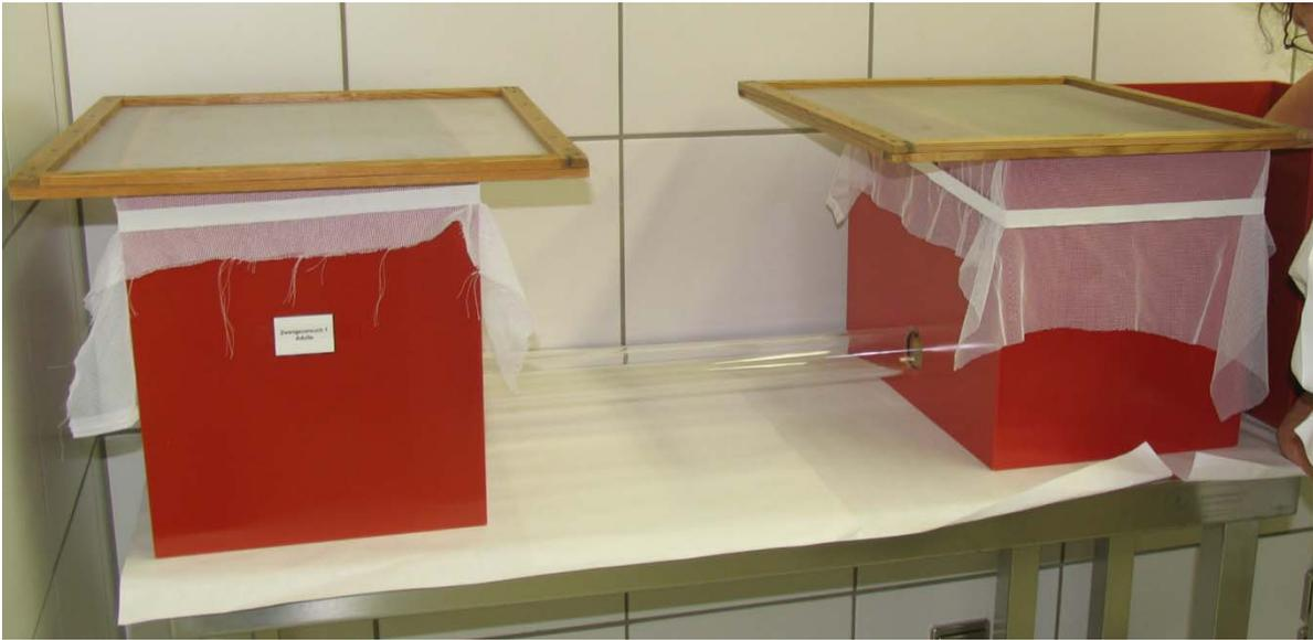
**Figure 1.** Arenas for testing cockroach baits: dual chamber box with rectangular units, side view
