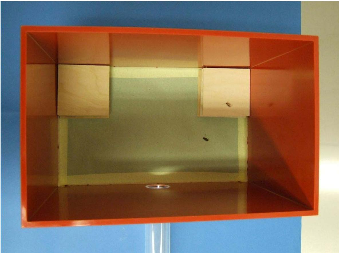
**Figure 2** Arenas for testing cockroach baits: harbourage unit of dual chamber box, top view
