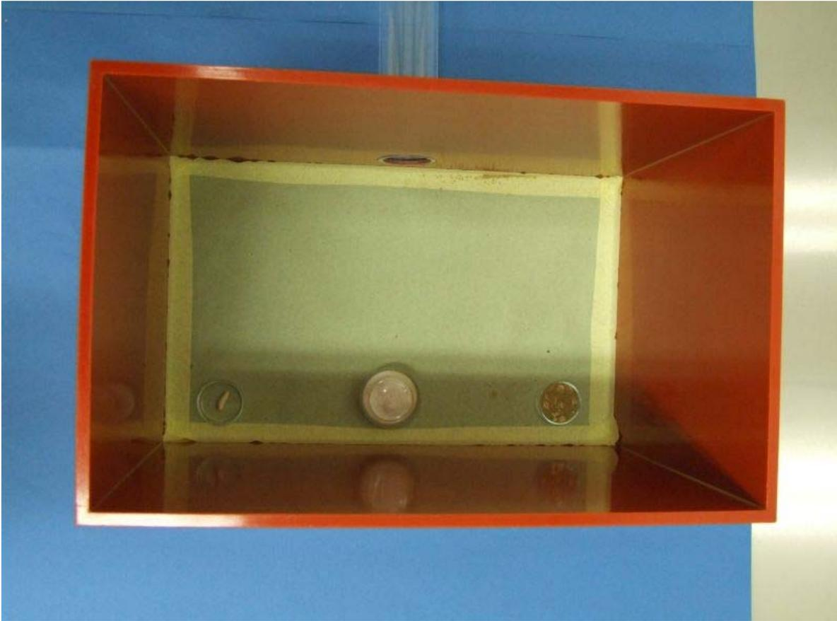
**Figure 3** Arenas for testing cockroach baits: feeding unit of dual chamber box, top view.
