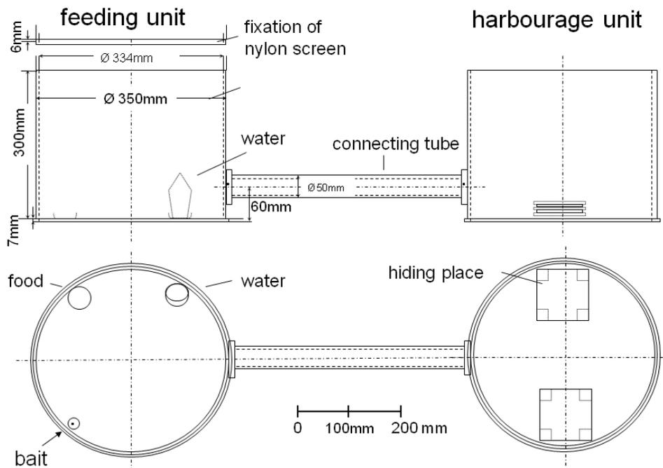
**Fig.4.** Arenas for testing cockroach baits: schematic representation of circular arenas, side and top views
