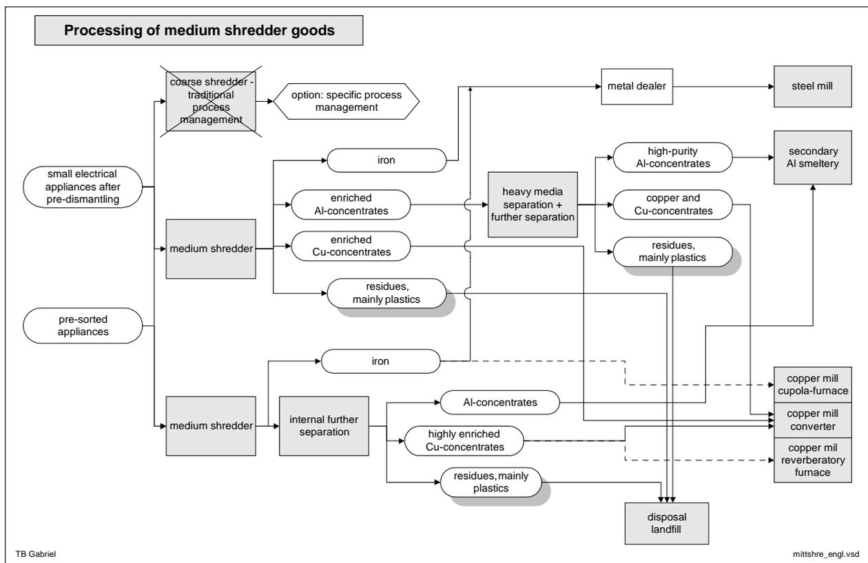
Fig. 1: Processing of medium shredder goods
