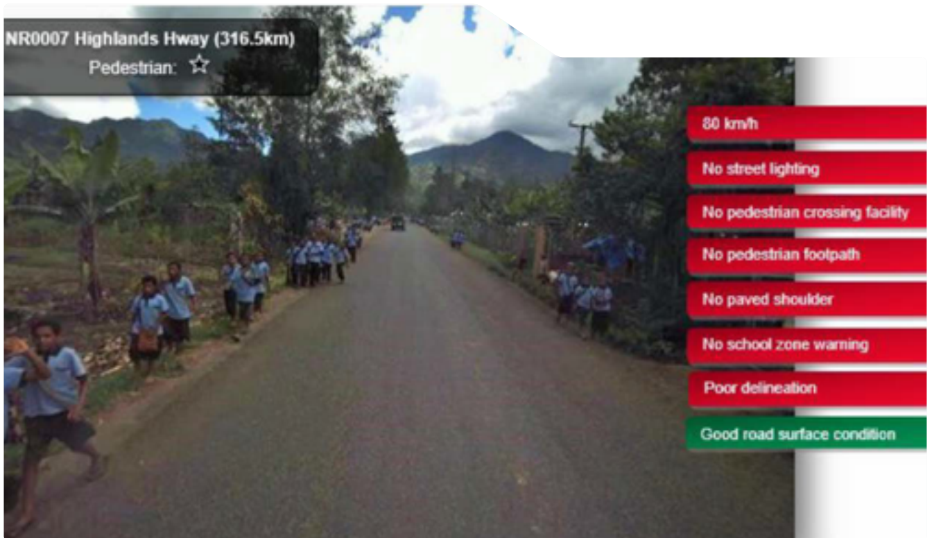
Example of a one star rated road for pedestrians; 97 per cent of the Highlands Highway has been assessed as being in this category.
