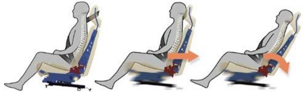
Autoliv/Volvo - WHIPS active whiplash protection
