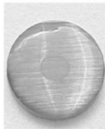
Figure 5 : Dried inoculum on carrier covered with 50 \mu\text{L} of test substance or control fluid
