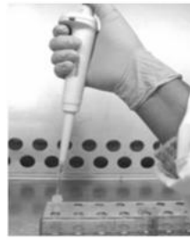
Figure 1 (left): Ten \mu\text{L} of the test organism inoculum being removed with a positive-displacement pipette
