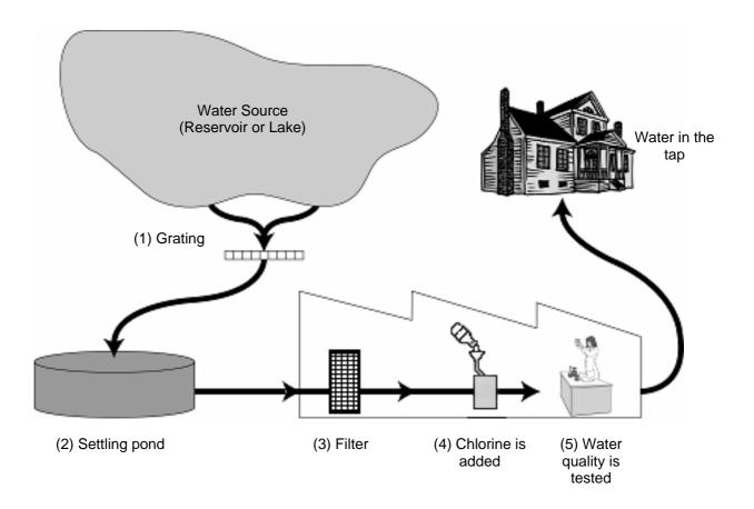
The figure above shows how water supplied to houses in cities is made fit for drinking.
