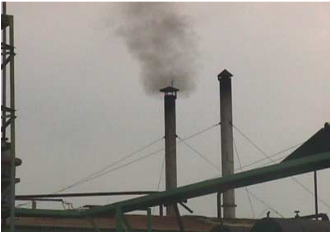
Photo 4: An industrial customer partially converted to gas. The left chimney still uses fuel oil while the right one uses natural gas (photo courtesy of PTT Natural Gas Distribution Co. Ltd. [PTTNGD]).
